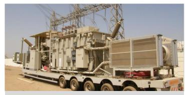
Mobile substation 154 kV, with transformer 40,000 kVA and set of equipment for 110, 35, 10, and 6 kV
